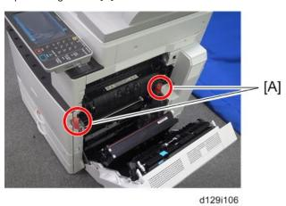
4. Remove the two stoppers [A] from the fusing unit.
