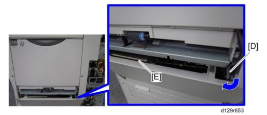
7. Push up the duplex unit a little bit, while pressing the bracket [D] to lock the spring [E].
